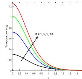
Fig. 2. Effects of  $M$  on temperature profiles
