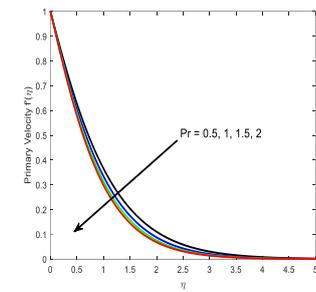
Fig. 4. Effects of  $Pr$  velocity profiles
