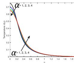
Fig. 15. Variation of temperature with variable thermal conductivity
